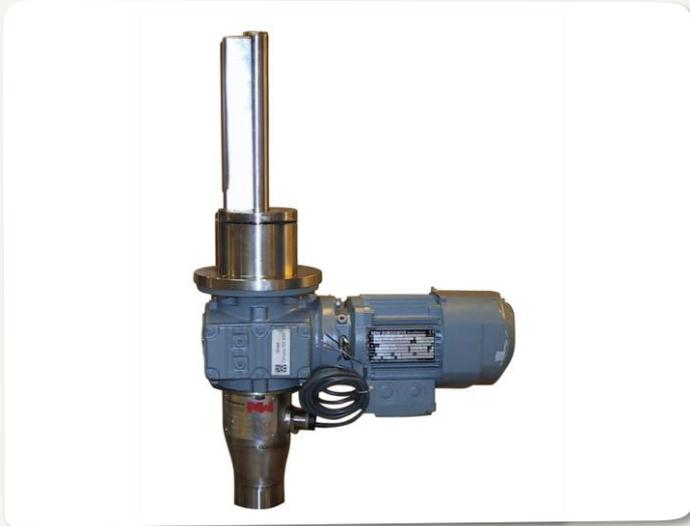
The Air Slide Sampler (AS) is designed for continuous or intermittent increment extraction of dry, non-sticky airborne powdered material ducted in horizontal or inclined air slides. The AS intersects ducted material, typically confined to a circular cross-section, in a linear increment transect.
