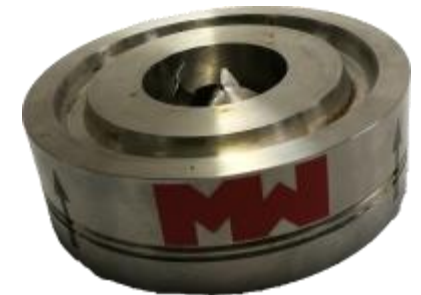
Ruptured burst disc after use
