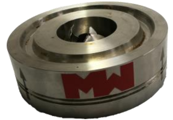
Ruptured burst disc after use
